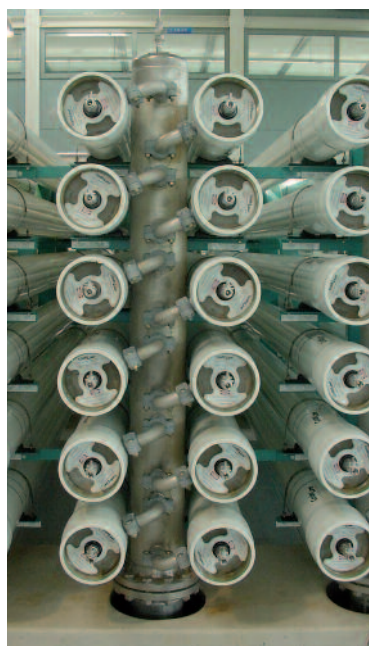
Desal membrane modules. Credit: Brent Alspach
