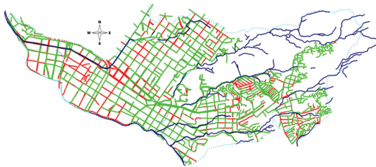
Figure 2 Schematic of the sections to replace and upgrade, showing the areas of greatest deterioration
