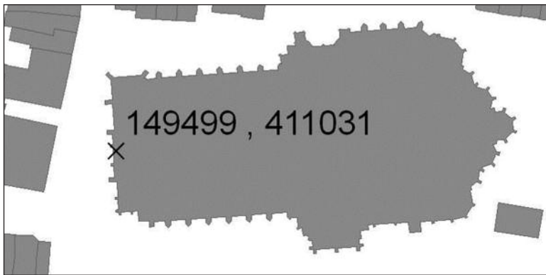
Figure 3 Difference in accuracy between a point object (x) and a polygon object
