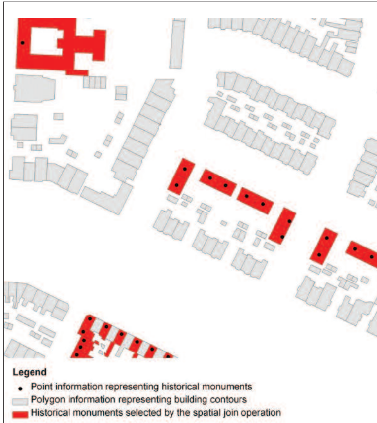
Figure 7 Selection of the pilot area. It appears that the data points of historical monuments match with the contours of buildings. The objects GIS selected as a monument using the spatial join operation are coloured red.
