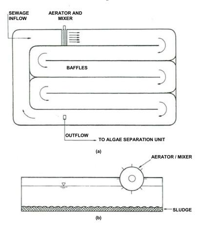
Figure 5.5 High-rate algal pond: (a) schematic plan, (b) schematic cross-section
