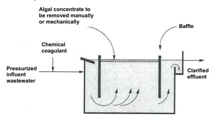
Figure 5.12 Schematic of a dissolved air flotation unit
