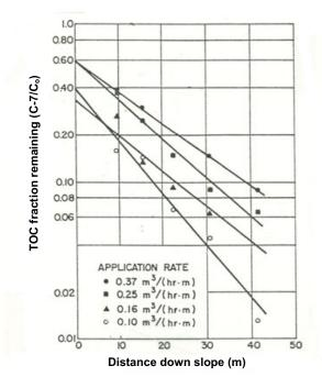
Figure 8.10 TOC fraction remaining versus distance down-slope; application rate study with screened raw wastewater (Smith and Schroeder 1985)
