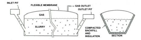
Figure 4.10 Plug-flow digester
