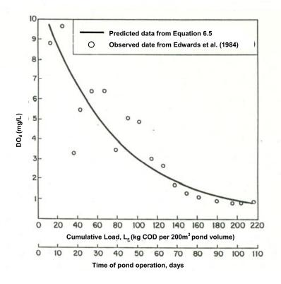
Figure 6.13 Cumulative load versus DO<sub>d</sub> for 100 kg COD/(ha-day) loaded septage ponds
