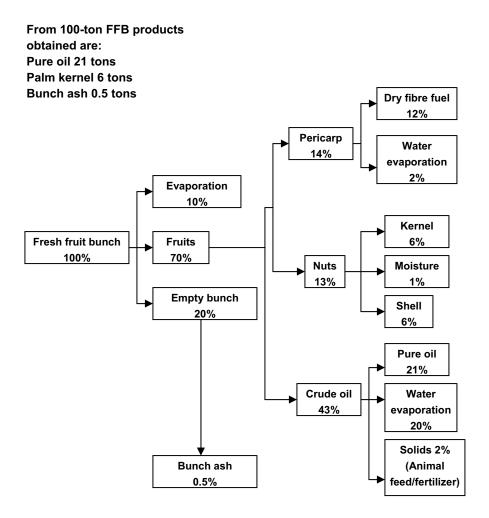
Figure 2.5 Product mass balance of a typical palm oil mill (Muttamara et al. 1987)
