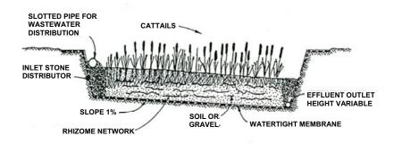
Figure 7.18 Typical cross-section of SF constructed wetlands (U.S. EPA 1988)
