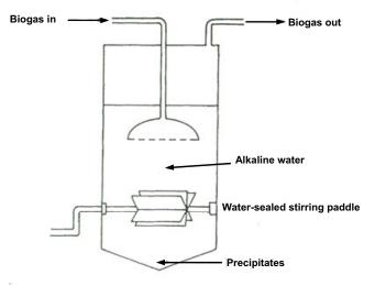
Figure 4.20 Model of CO2 and H2S scrubber in alkaline water
