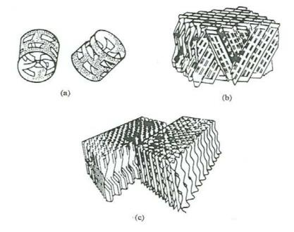
Figure 4.15 Packing media for anaerobic filters: (a) pall ring; (b) crossflow media; (c) tubular media
