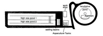
Figure 5.8 Advance integrated wastewater ponding system (Pilot plant at the University of California, Berkeley, Richmond Field Station, USA)
