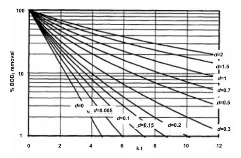
Figure 7.14 Design chart for BOD<sub>5</sub> removal in water hyacinth ponds (Polprasert *et al.* 1998)
