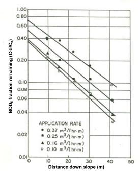
Figure 8.9 BOD<sub>5</sub> fraction remaining versus distance down-slope; application rate study with screened raw wastewater (Smith and Schroeder 1985)
