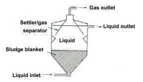
Figure 4.16 Upflow anaerobic sludge blanket digester
