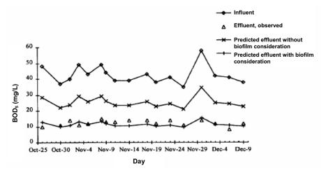
Figure 7.13 Predicted and observed effluent BOD<sub>5</sub> concentration of the WHP (Polprasert and Khatiwada 1998)
