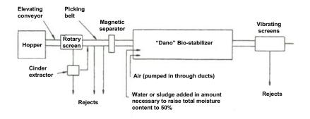
Figure 3.17 Typical DANO plant (after Flintoff and Millard 1969)
