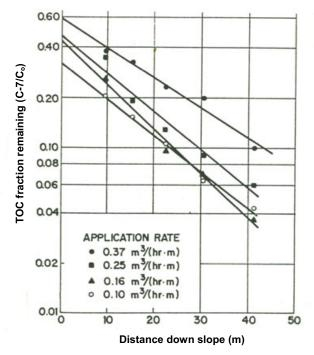
Figure 8.12 TOC fraction remaining versus distance down-slope; application rate study with primary effluent (from Smith and Schroeder 1985; reproduced by permission of the Water Pollution Control Federation, USA)
