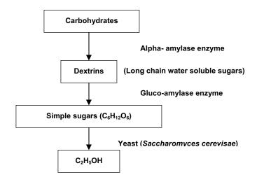
Figure 4.23 Ethanol production process
