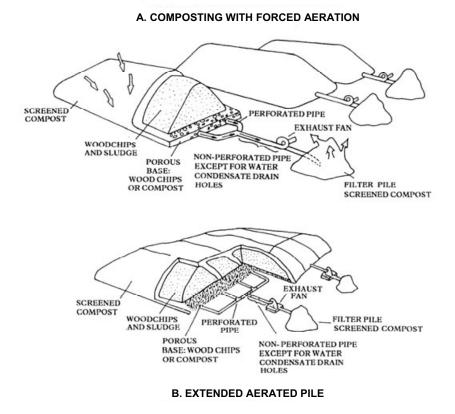
Figure 3.14 Configuration of aerated piles showing construction of pile and the arrangement of aeration pipe - the BARC system (Shuval *et al.* 1981; reproduced by permission of the World Bank)
