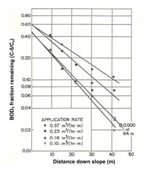
Figure 8.11 BOD<sub>5</sub> fraction remaining versus distance down-slope; application rate study with primary effluent (Smith and Schroeder 1985)
