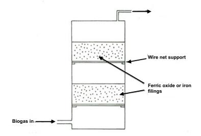
Figure 4.21 Model of dry gas scrubber for H<sub>2</sub>S removal
