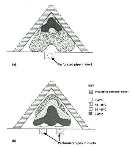
Figure 3.16 Typical temperature cross-section distributions in a pile with (a) positive pressure (blowing) aeration; and (b) negative pressure (sucking) aeration (from Stentiford *et al.* 1985; by permission of the Institute of Water Pollution Control, U.K.)
