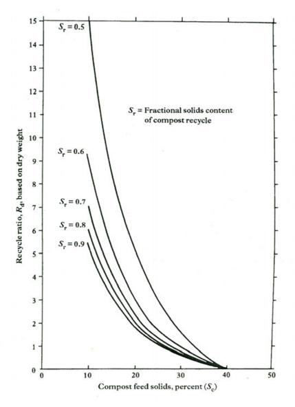
Figure 3.6 Effect of compost feed solids content on the dry-weight recycle ratio needed to achieve a 40 percent mixture solids content (Haug 1979; reproduced by permission of the Water Pollution Control Federation USA)
