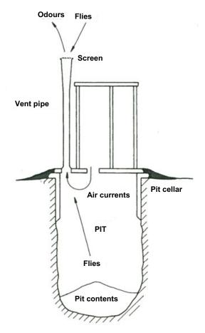
Figure 3.9 Schematic diagram of a ventilated improved pit latrine (Morgan and Mara 1982; reproduced by permission of the World Bank)
