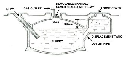
Figure 4.5 Fixed-dome digester
