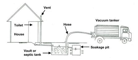
Figure 2.1 Vacuum tanker removing septage
