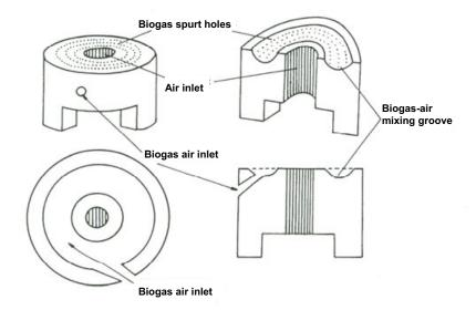
a) Earthen stove with mixing groove
