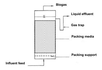
Figure 4.14 Up-flow anaerobic filter
