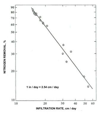
Figure 8.8 Effect of infiltration rate on nitrogen removal for rapid infiltration, Phoenix, Arizona (From Lance and Gerba 1977; reproduced by the permission of Pergamon Books Ltd)
