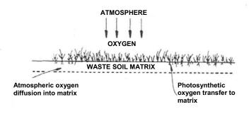
Figure 8.7 Schematic of oxygen transfer to stabilize organic compounds applied to land
